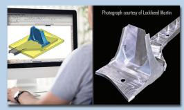
Starting with a 3D model from a CAD program, Sciaky's fully-articulated, moving electron beam gun deposits metal (via wire feedstock), layer by layer, until the part is built and ready for finish machining. Deposition rates typically range from 7 to 20 lbs/hr (3 to 9 kg/hr), depending upon part geometry and the material selected.
